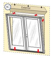
D. Plumb and square door. Place shims at each hinge and lock strike location between the door and the sides of the opening. Insert shims in other locations as needed starting up 6" from the bottom of the door to square it in the opening. Make sure that the reveal around the door(s) is equal. On double doors, make sure that panels are even across the bottom.
